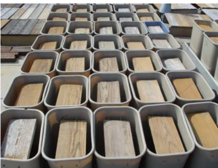
Figure 1b Figure 1: Treated and coated deck boards (a) newly installed; (b) After 3 years natural weathering
