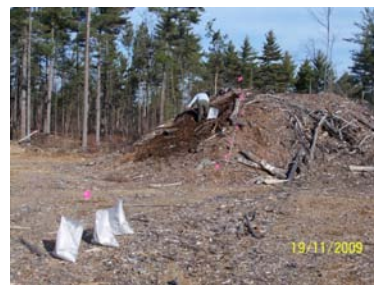
Digging a deep hole in a pile, the tape running up the side, with those pink flags, extends 7+ m.
