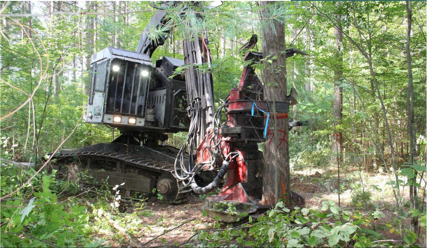
A feller-buncher thins a plantation in the United Counties of Prescott and Russell's FSC certified Larose Forest. Ensuring harvests are sustainable is an important part of FSC certification.
