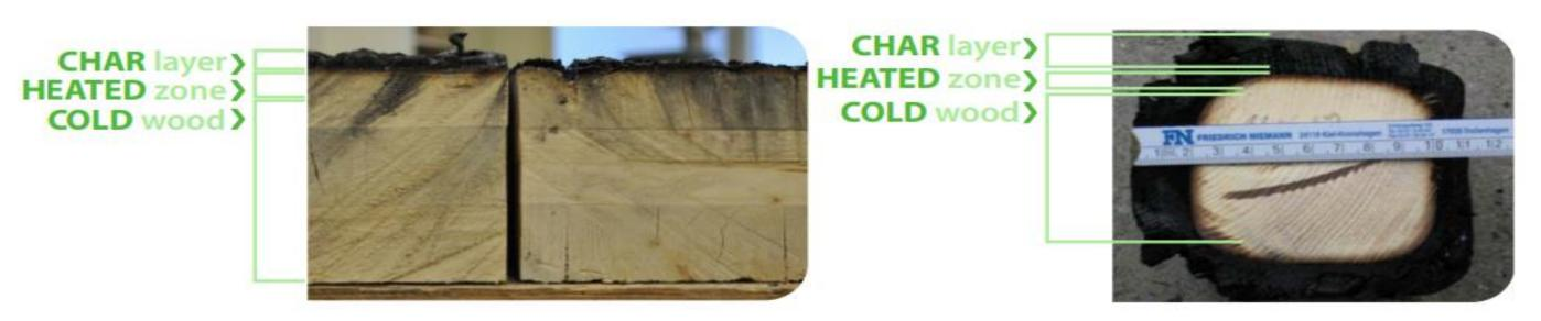
The unburnt wood, protected by the charred wood, retains up to 100 percent of its initial strength.
