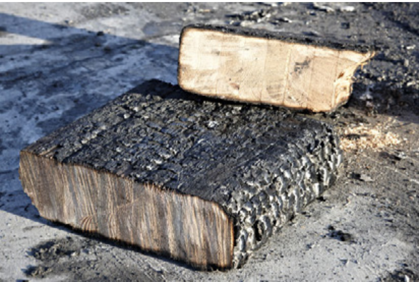
Mass timber is a combustible material that provides impressive fire safety. During fires, exposed mass timber chars on the outside, which forms an insulating layer protecting interior wood from damage. Additionally, when the code requires mass timber to be protected with gypsum wall board, fire testing indicates it can deliver much higher than required fire ratings.
