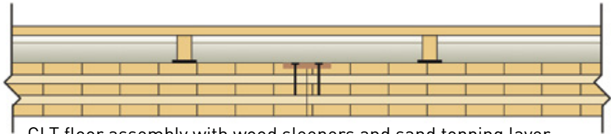
CLT floor assembly with wood sleepers and sand topping layer. (Note the isolation gasket between the sleepers and the CLT panel. Membrane required to prevent sand leaking through gaps in CLT.)
