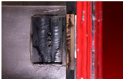
Wood joining by linear friction welding. Image Credit: TWI Ltd.
