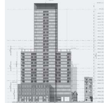
2022 [Proposed] redevelopment of the site with a 30-storey mixed-use building with retail at-grade along Spadina Avenue and 550 dwelling units above. East Elevation. Wallman Architects. Supporting Documentation, City of Toronto Official Plan and Zoning By-law Amendment Application. July, 2022, 1/A.4.02.
