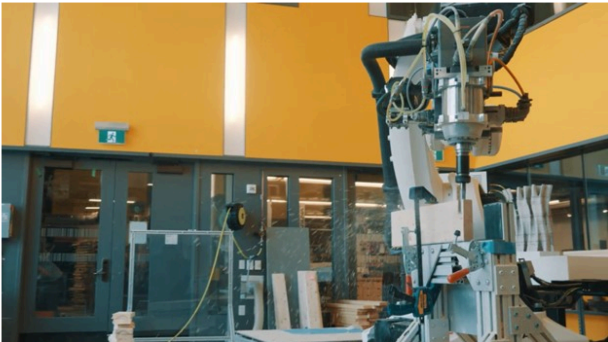
Image: KUKA 5-axis robot milling a piece of wood at the Daniels Robotic Facility at UofT. Credit: Six Films
