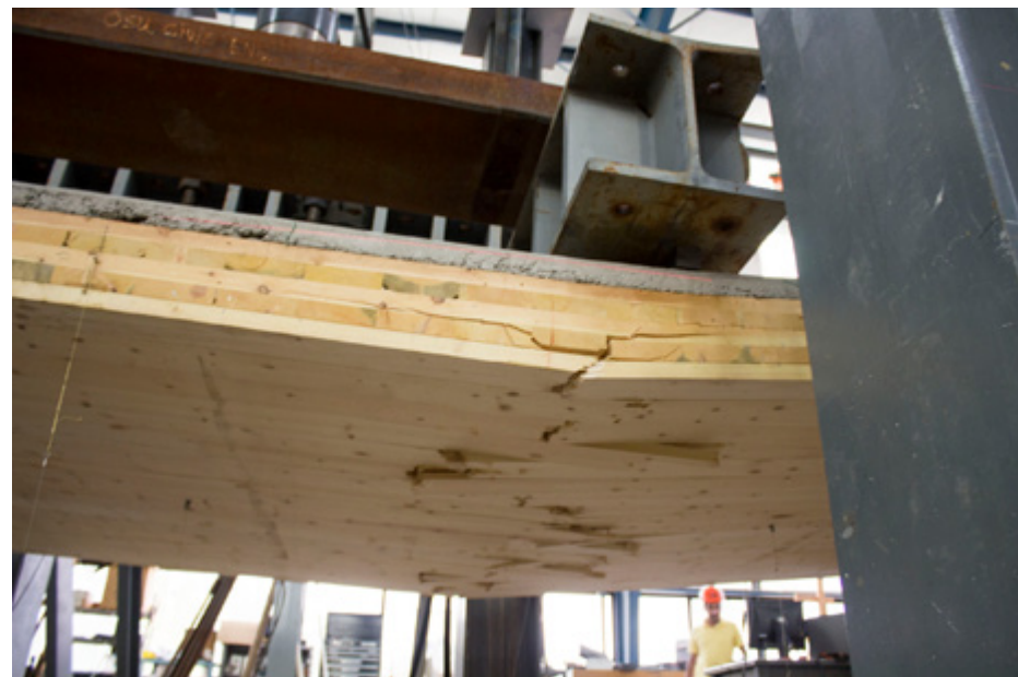
Testing timber concrete composite assemblies. The use of TCC assemblies addresses a number of structural, acoustical and fire safety issues in mass timber buildings. A great deal of research into the performance various TCC technologies is running parallel to the development of reliable design methods. (Oregon State University)
