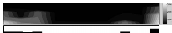
Figure 1: Workplane illuminance indicating high variation (scale in lux) (top) and corresponding shade positions (bottom) (white means shade closed)
