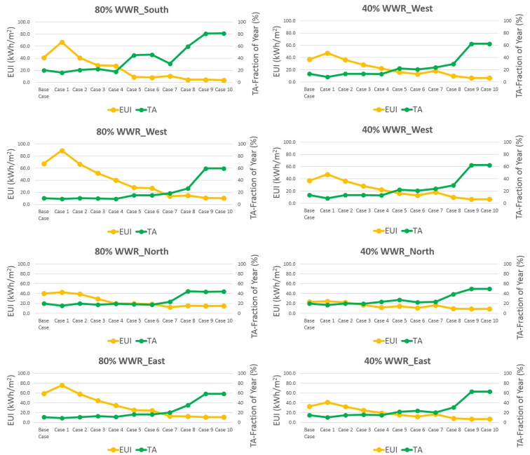
Figure 7. Sensitivity of EUI and TA to design alternatives in different scenarios and orientations.
