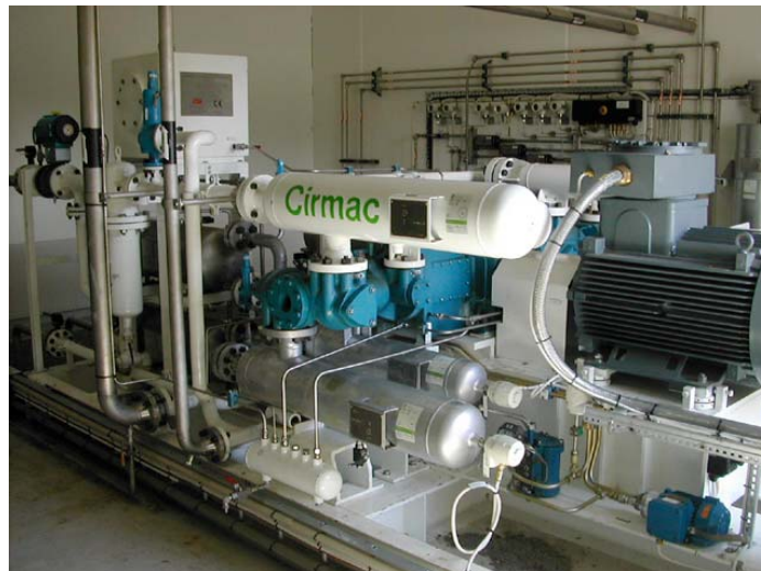
Figure 44. Biogas conversion into pipeline quality natural gas (methane) is a high technology industry that has the potential to create research expertise and new manufacturing jobs in Ontario. [Photo courtesy Cirmac, Sweden]
